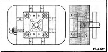
Fig. 46. Die-bed for Sectional or Split Dies
